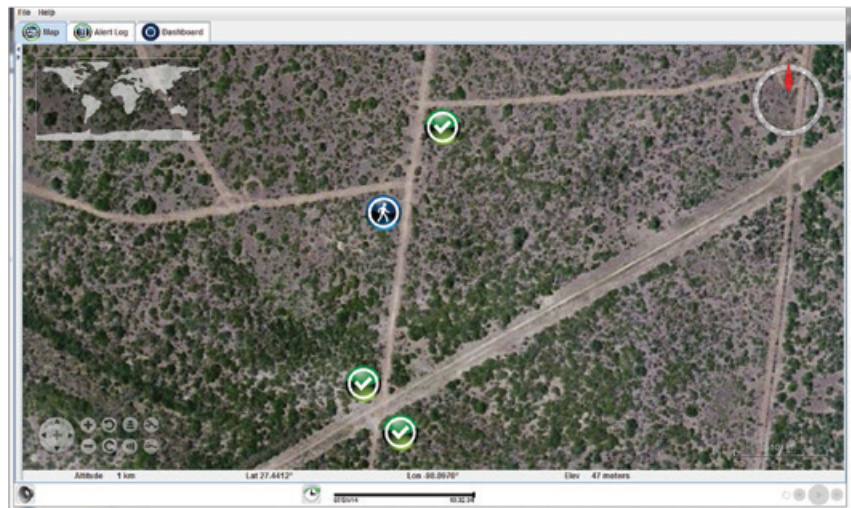
User interface view, showing footsteps detection & classification by sensor #3
