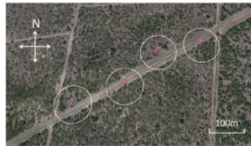
Sensor placement along pipeline. Sensors are placed on either side of the pipeline for better coverage. The 50 meter radius white circles are for distance visualization only.
