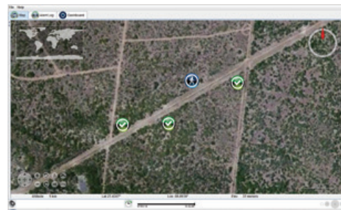
Screen shot of the user interface. At this point, sensor #3 is alerting. Sensors #1 and #2 have already alerted, and sensor #4 will alert as the walker continues NE along the pipeline.
